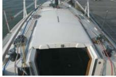
Above: The sail control lines are handled on either side of the companionway, seen here without the sprayhood fitted
