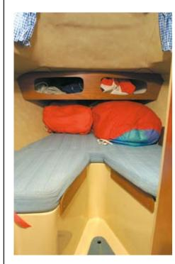
Above: The forecabin offers two vee berths of just under 6ft, which can be converted to a double with an infill board between the berths
